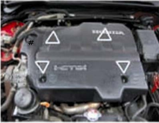
UNDO THE 4X10 mm FIXING NUTS
